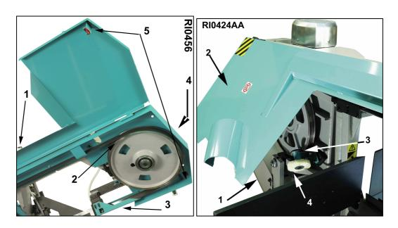
Make sure that there are no chips or dirt on the pulleys, and following the cutting direction, shown also by an arrow, put the new blade in the guides **without removing the plastic protection**, and then on the pulleys. The upper supports prevent the blade from falling. Tighten the tension-adjusting screw and make sure the blade is correctly placed on the pulleys. **Remove the plastic protection**, then assemble the blade guard and the front mobile protections.
