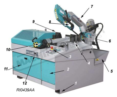
If not tensioned : stretch the springs.-6/RI0439 - placed at the back side of the machine to balance the saw frame : loosen the fixing springs of the sliding plate - and, by a lever , place it about the half of the slots. Hardly lock the screws immediately. It is necessary to do these operations with the saw frame completely up.
