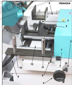
Therefore level the loading roller table to the same level of the work table and the back supporting jaws by beginning to that nearest the machine. For very long workpieces adhere the pedestals on the floor and
